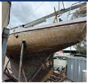
This resulted in Thara being sailed to Sydney to remove the mast and crane her out onto a truck, thence to a boat storage yard at Huskisson where the investigation could be continued more thoroughly without the time and cost pressure of a dockyard hardstand. The stem has been removed and the hull soda-blasted to expose any damaged timbers, loose fasteners and facilitate re-caulking to stop (or at least, reduce) the inevitable leakage.
