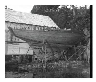
The boat is 10.5m long (34ft), narrow beamed at just over 2m, draws 1.6m and weighs 6 tons with a 13m aluminium mast, Bermudian rigged.
